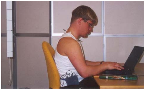
Fig. 3. Conventional laptop, test situation B = The subjects place the laptop computer on the tabletop surface and adjust the VDT screen tilt to their preference.
