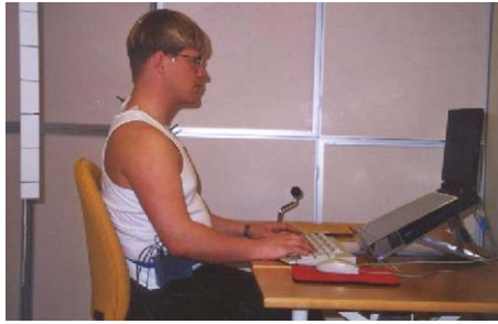
Fig. 2. ErgoQ Laptopstation, test situation A = The subjects adjust the keyboard, VDT screen height, tilt and distance to their preference and comfort, following instructions on the adjustability of the ErgoQ laptopstation.
